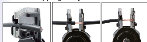
First Stripping Second Stripping (For both First and Second Stripping)
